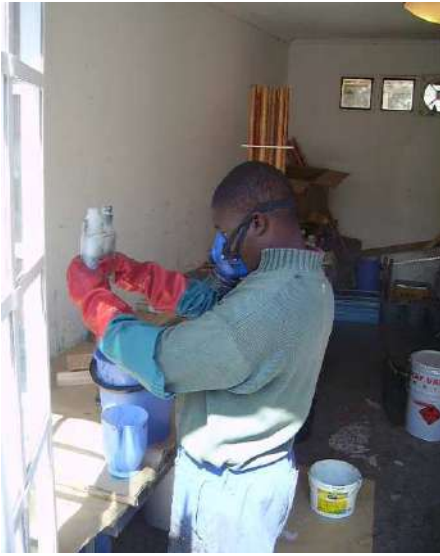
Measure the needed quantity of catalyst
