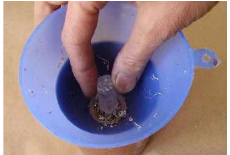
Place top crystal into nest with tip facing downwards (up in finished HHG)
