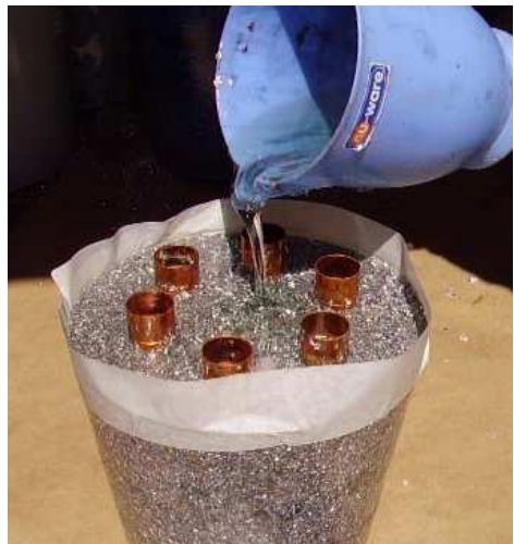
Pouring a smooth top coating with tape
