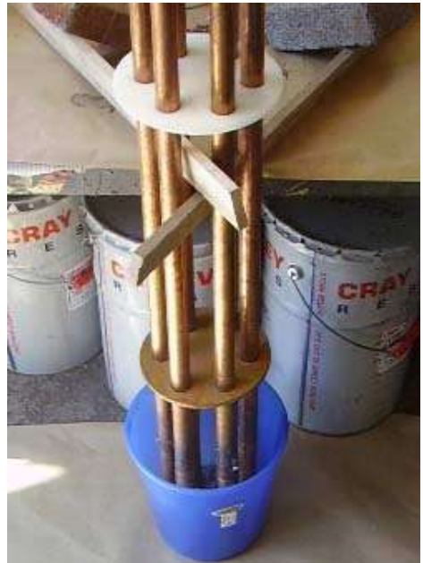
Apply some preliminary bracing
